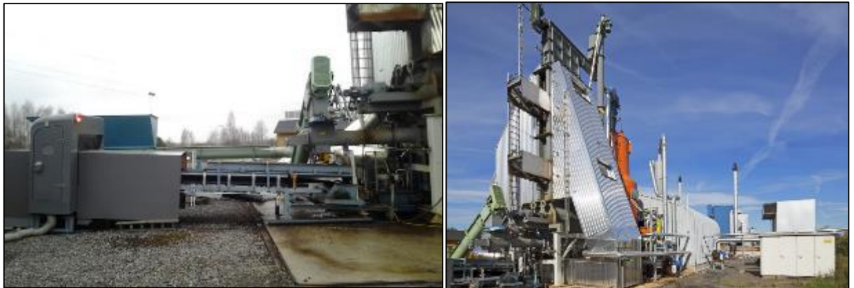
Picture 1 Inray Fuel x-ray scanner installed in belt conveyor in Torrec Oy's biocoal plant
